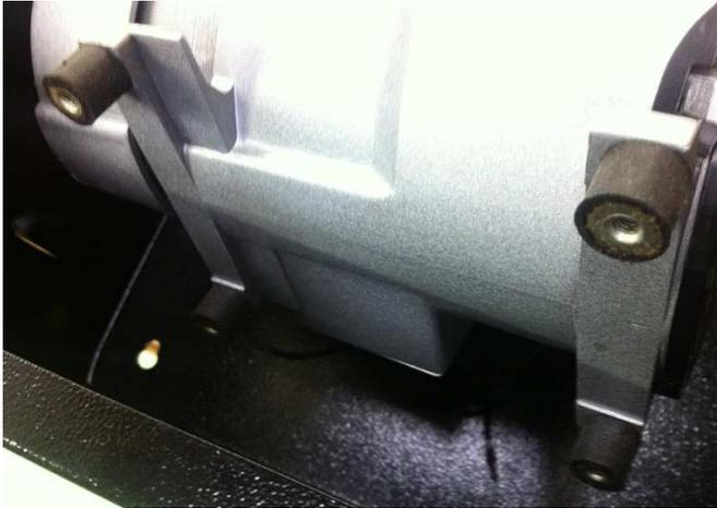
5. Install smaller screws into the vibration absorbing feet. **Do not over tighten screws!**
